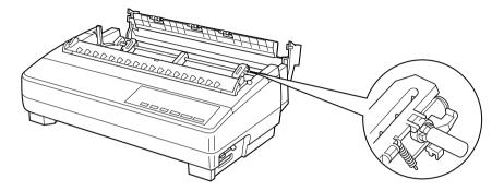
☐ Before printing, make sure that the leading edge of the fanfold paper extends about 0.8 inch (two centimeters) past the front the paper chute, as shown in the illustration below.
