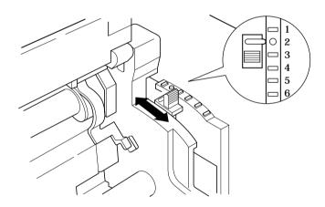
☐ Move the adjustment lever to one of its four settings. Position 2 is most suitable for single-sheet paper.
