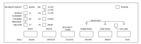
This chapter describes control panel functions that can be performed while the printer is turned on and either on-line or off-line. The buttons perform different functions in the EDS and Dot Adjustment Modes. Functions of control panel buttons in these modes are described in the relevant sections covering them.
