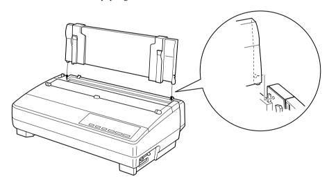
☐ To remove the paper guide from the printer, simply pull the tabs out of the holes.
