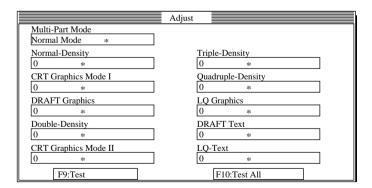
Use the above window to test and adjust the vertical alignment of the printer in each printing mode. See "Adjusting the dot alignment" on page 72 for full details on dot alignment.
