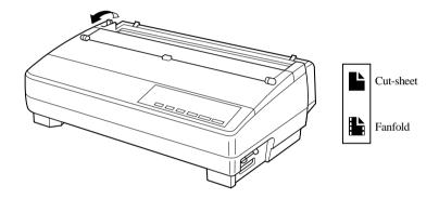
Grasping the two back corners of the printer with the palms of your hands, press back on the two raised areas on the top of the rear cover until it opens.
